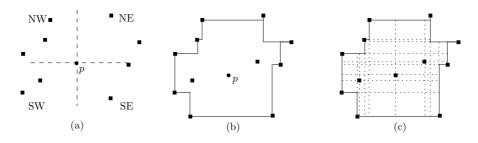
Figure 2: (a) Point p is orthogonally well illuminated because all oriented quadrants centered at p are non-empty. (b) Point p is interior to the orthogonal convex hull of F, so it is orthogonally well illuminated. (c) An orthogonal convex hull decomposed into several rectangles.
