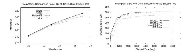
Figure 7: Number of tpmC-uva using different number of warehouses for each file system considered (left) and maximum throughput of the New Order transaction in each case (right).
