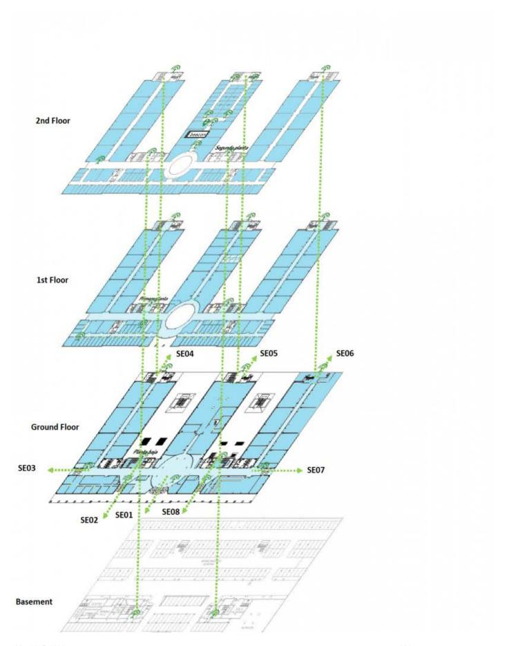
Figure: representation of building and antennas
